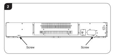
2.10 Unhook the wall mounting bracket from the appliance.
