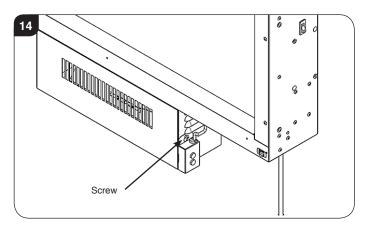
4.14 Remove the 2 screws from the front of the appliance, see Diagram 15.
