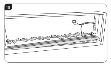
9.4 Replace in reverse order. NOTE: The flexible fuel bed locates in a groove in the bracket, see Diagram 16.
