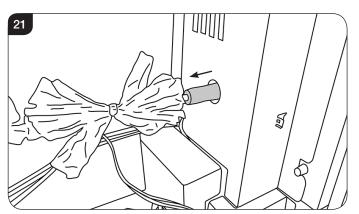
12.4 Gently withdraw the spindle from the support brackets at an angle, see Diagram 22.
