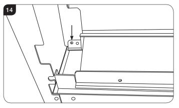
9.3 The bracket and the Fuel Bed can now be lifted out of the appliance, see Diagram 15.
