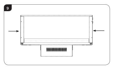
8.2 Remove the screws that secure the side panels, see Diagram 10.
