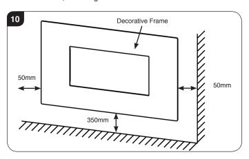
4.2 Decide on the height from the floor level to the bottom of the recess opening (minimum of 350mm).
