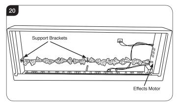
12.3 The Effects Spindle is attached to the Effects Motor by a rubber sleeve.
