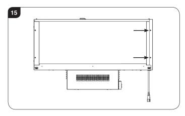
4.15 Remove the 2 screws from the rear of the appliance, see Diagram 16.
