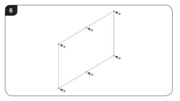
3.8 Attach the bracket to the wall using the screws provided ensuring the hooks are at the top, see Diagram 7.
