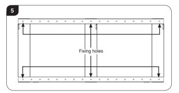
3.7 Drill the holes and insert the rawlplugs provided. Note: The rawlplugs supplied are suitable for solid wall applications. If it is intended to mount the appliance onto plasterboard or hollow walls suitable fixings must be used, see Diagram 6.
