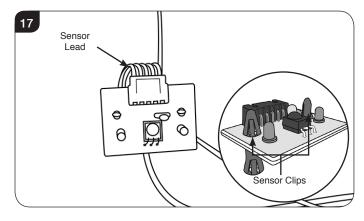
10.4 Remove the sensor and replace as required.
