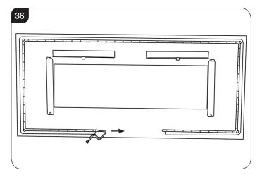
18.3 Carefully withdraw the LED strip from the channel, see Diagram 37.
