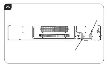
5b.4 Attach the connector to the hardwiring kit.
