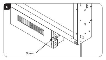
7.3 The Heater Unit is attached to the bottom of the appliance by 4 screws, see Diagram 7.
